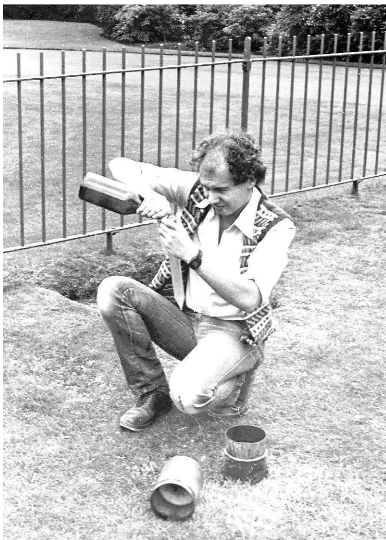
Figure 24 Steve Garland taking measurements of rainfall from the 5" raingauge, 1982 (© Museums Sheffield)
