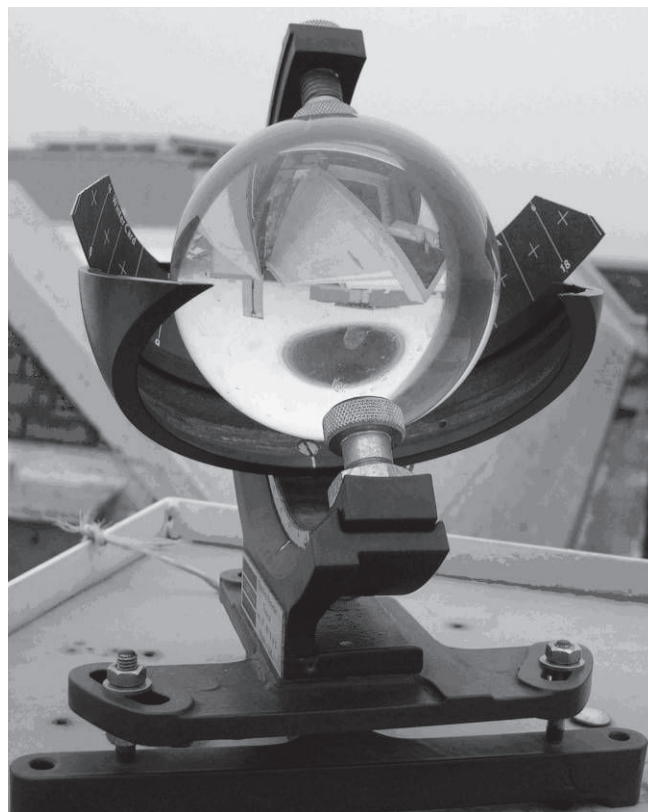
Figure 34 Campbell-Stokes sunshine recorder with locking nuts (courtesy of Museums Sheffield)
