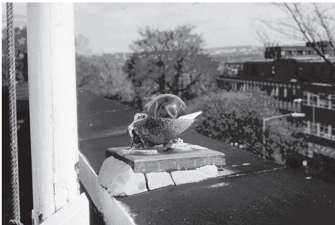
Figure 32 Campbell Stokes sunshine recorder sited above the entrance to the museum circa.1900's to 1996 (© Museums Sheffield)
