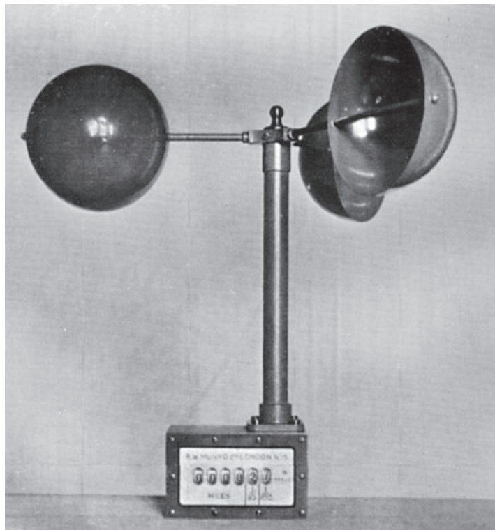
Figure 12 Robinson three cup anemometer (from Meteorological Office 'The Observer's Handbook' 1934)
