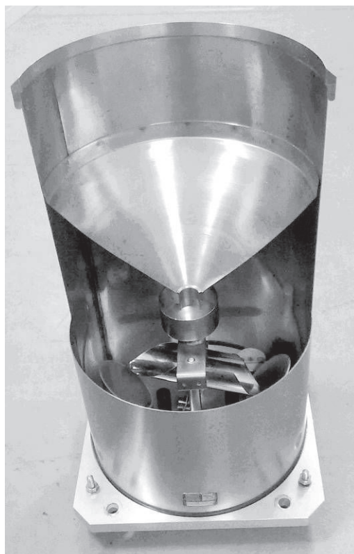
Figure 36 Tipping bucket rain gauge, part cut away to reveal tipping bucket mechanism beneath collecting funnel (courtesy of Museums Sheffield)
